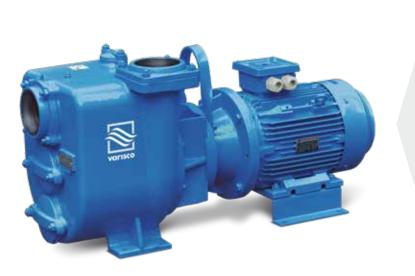
Suction port Threaded - 3" ISO 228 (BSP) Delivery port Threaded - 3" ISO 228 (BSP) Qmax 70 m<sup>3</sup>/h - 1166 l/min (308 USgpm) Hmax 66 m (216 ft) Solids handling 14 mm (0,55") Motor power 18,5 kW - 25 HP Motor brand Electroadda E3G Weight 240 kg (529 lb)
